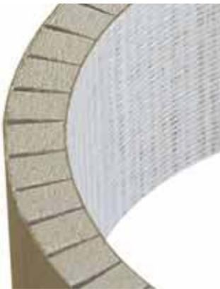
**Our modern manufacturing equipment has the facility to cut not just V grooves but also slots into the plasterboard.** This enables the manufacture of curved on section profiles such as round column casings, curved ceiling bulkheads, curved walls/linings or rounded end caps for partition walls.
